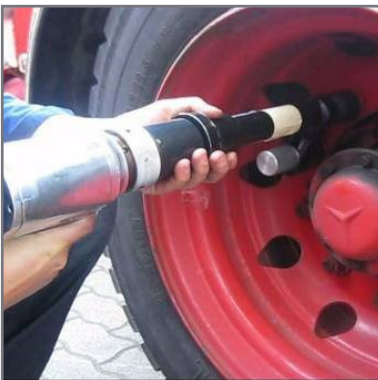
The easily adjustable cup rests on a nearby nut and prevents damage to the rim.
