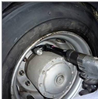
With the HYTORC Wheelgun Arm, deep-lying wheel bolts are also easily accessible.
