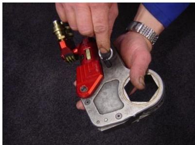
3. Finally, you replace the safety pin. After changing the ratchet, you have to test if the hexagon of the tool turns and everything operates as desired, before placing the tool on the nut.
