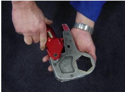
2. Next, you slide the cylinder in another ratchet and ensure that the safety pin holes of cylinder and ratchet are in line.
