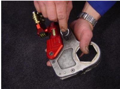
1. Firmly hold the hydraulic cylinder and pull out the safety pin. Now you can take off the ratchet from the driving cylinder.
