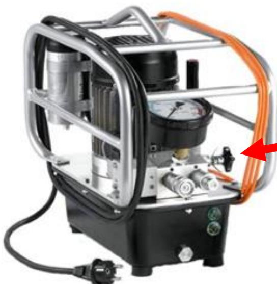
6. Turn the wing nut to the right until the pressure gauge presents the desirable pressure. After setting, you can release the start button.
