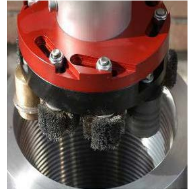
Mechanical cleaning of internal thread with different brushes.
