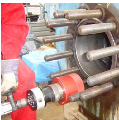
BoltClean in action. Studbolts and bolts are cleaned quickly and easily.
