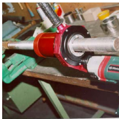
A BoltClean with lateral drive for the complete cleaning of long studbolts.
